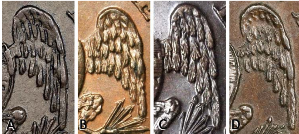
Figure 5. Close-up images of the left wings of the four reverses. None of the wings match, demonstrating that they were not produced from the same hub.
